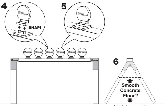
Add chains or rope to keep legs from sliding out. (Chains/Rope - Not Included with Alpha Brackets.)
